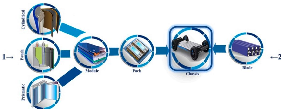
**Fig. 13.** EV battery production steps: (1) conventional cell, module, pack, and chassis route for NMC and NCA chemistries versus (2) cell-to-chassis design for large format LFP cells. Reproduced with permission from [231].
