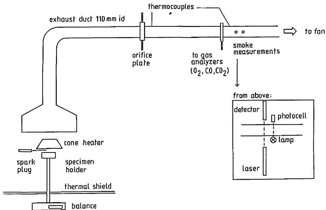
Figure 1. Cone Calorimeter.
