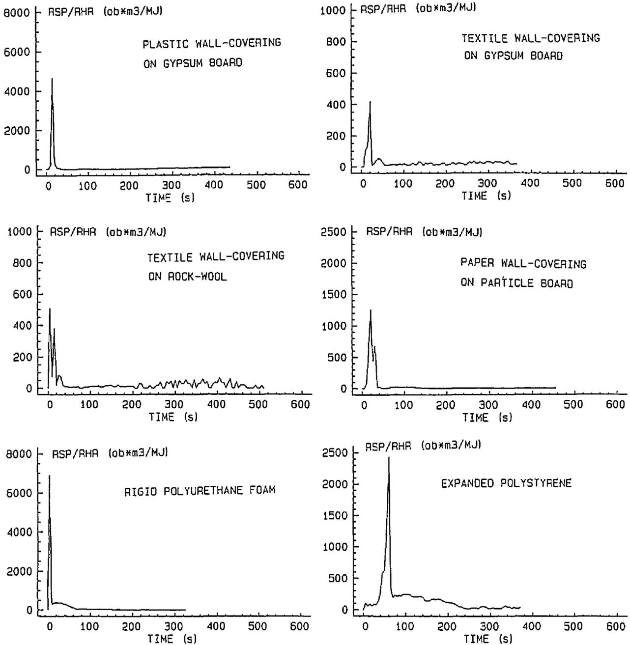
Figure 16. The rate of smoke production (RSP) divided by the rate of heat release (RHR) at  $50 \text{ kW/m}^2$  for the 13 building products. Note the different scales.
