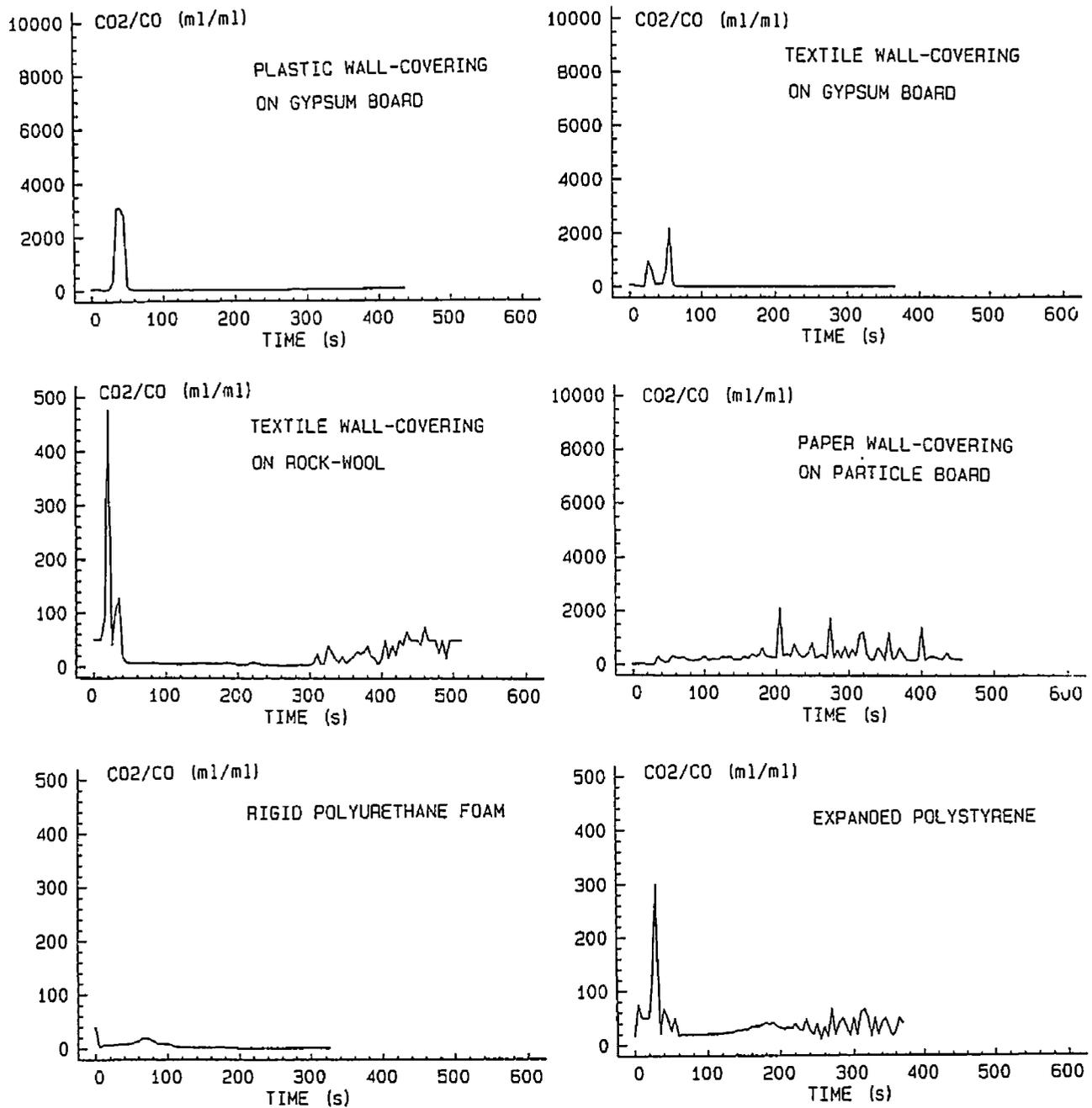
Figure 18. The carbon dioxide production ( $\text{CO}_2$ ) divided by the carbon monoxide production ( $\text{CO}$ ) at  $50 \text{ kW/m}^2$  for the 13 building products. Note the different scales.
