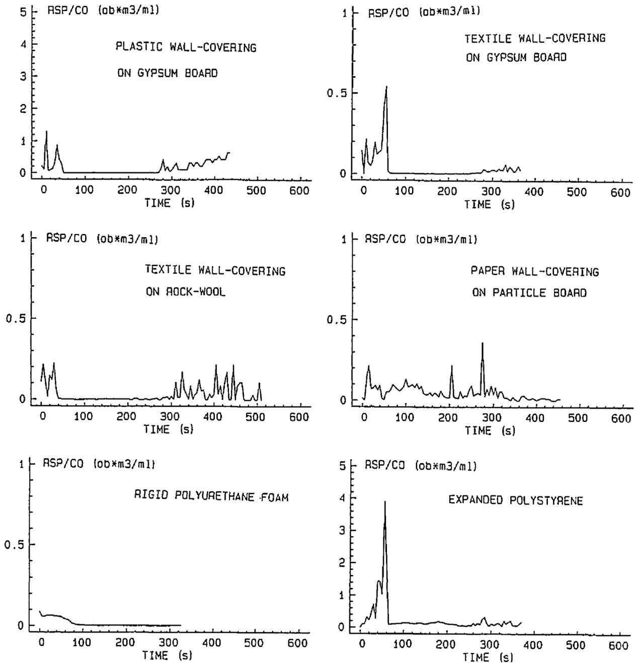
Figure 17. The rate of smoke production (RSP) divided by the carbon monoxide production (CO) at  $50 \text{ kW/m}^2$  for the 13 building products. Note the different scales.
