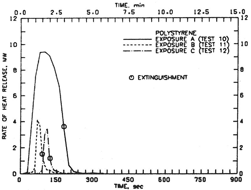
FIG. 3—Rate of heat release history for polystyrene.
