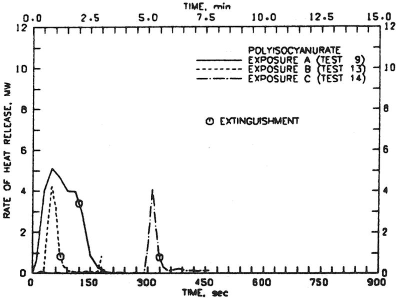
FIG. 4—Rate of heat release history for polyisocyanurate.
