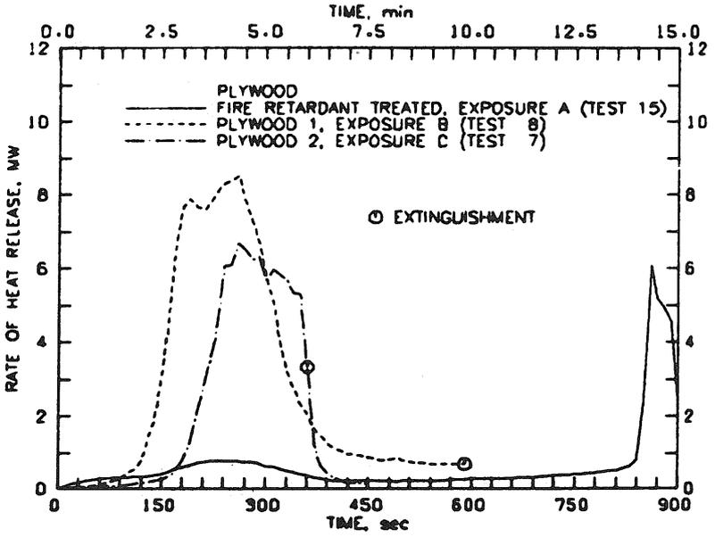
FIG. 2—Rate of heat release history for plywood.
