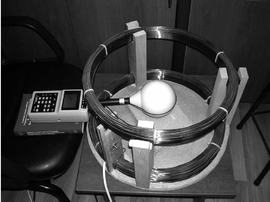
**Fig. 3.** Magnetic Field Exposure System
