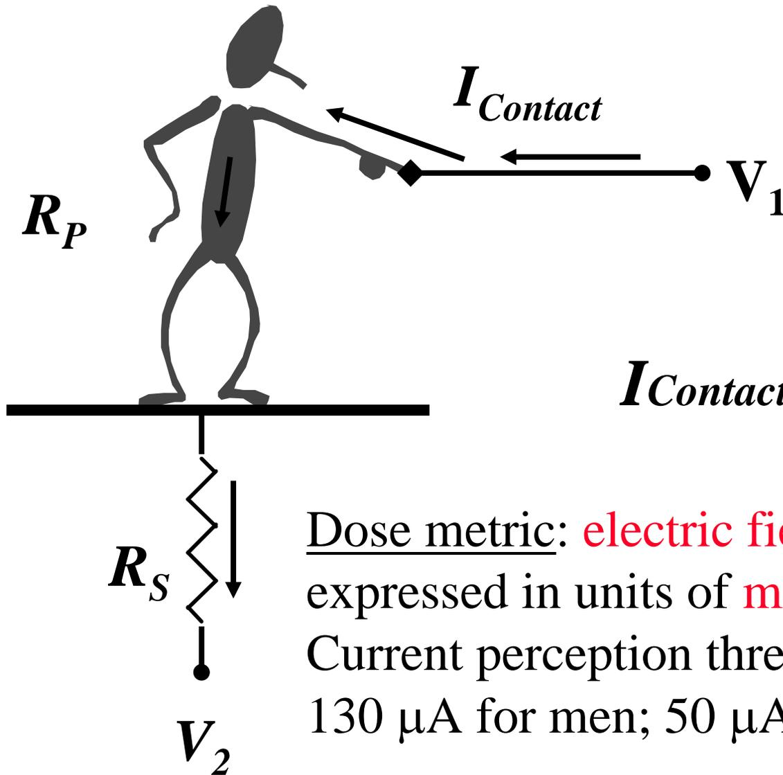
$$I_{Contact} = \frac{V_1 - V_2}{R_P + R_S}$$
