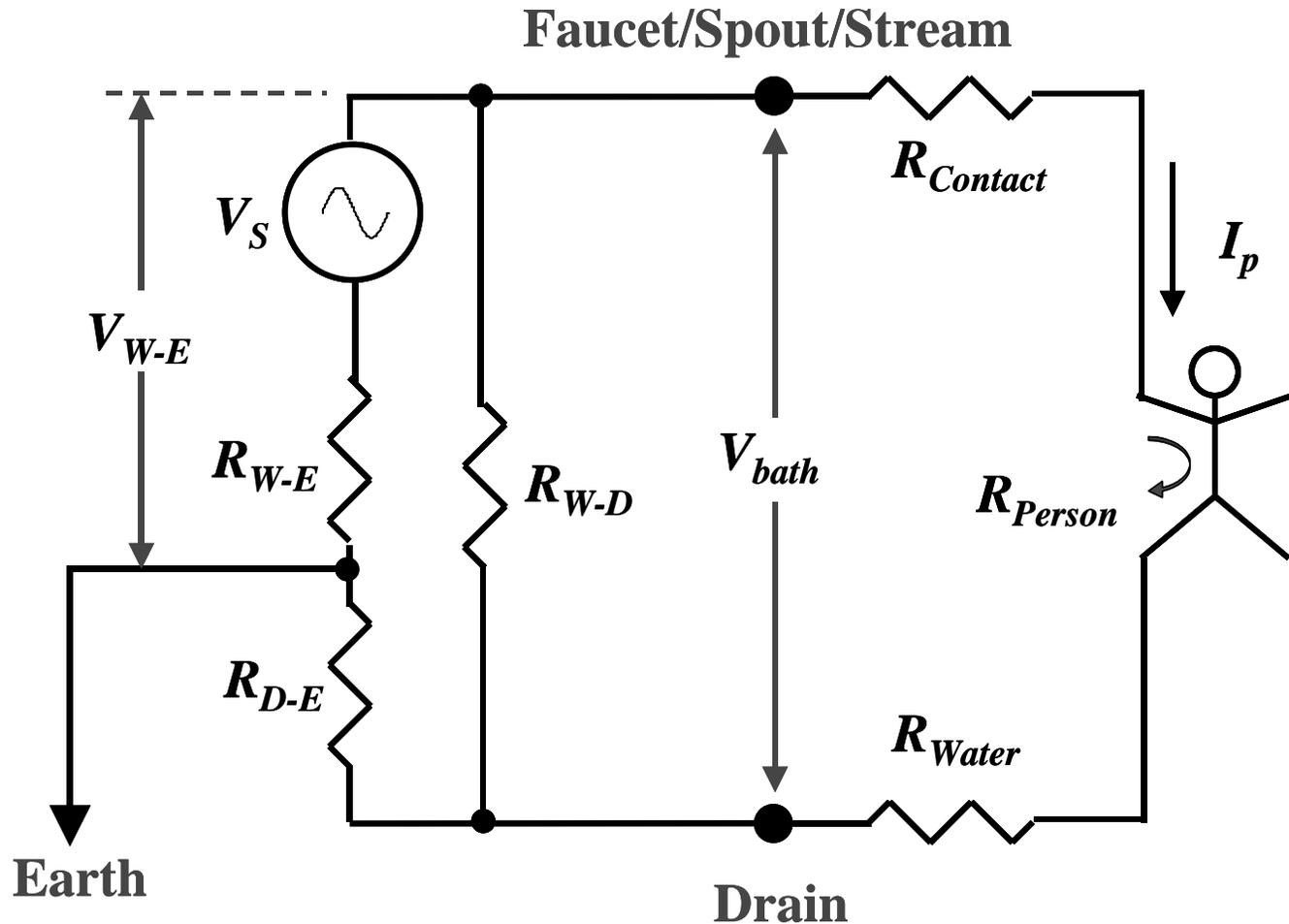
$V_{bath}$  is a variable fraction of  $V_{W-E}$  depending on soil conditions and relative positioning of drain and water lines;  $V_{bath}$  negligible if either drain or residential water pipe is non conductive
