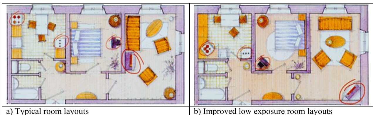
Figure 3. Inappropriate layouts/specification may increase both field and contaminant exposures [20]. (Reproduced with kind permission from the Russian National Committee of Non-Ionising Radiation Protection).
